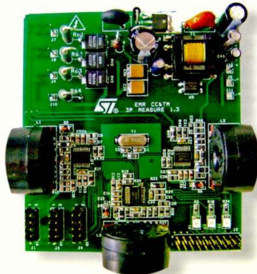
3-Phase energy meter measurement module STPM01 based
